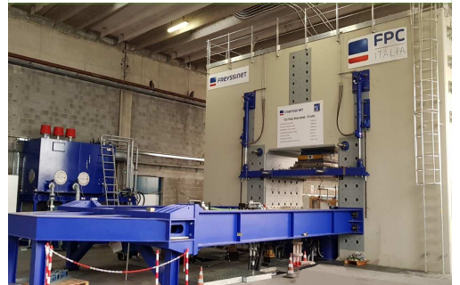
Figure 2. 70 MN Testing Bench at ISOLAB.
