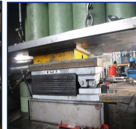
50 MN Press "Horizontal capacity test"
