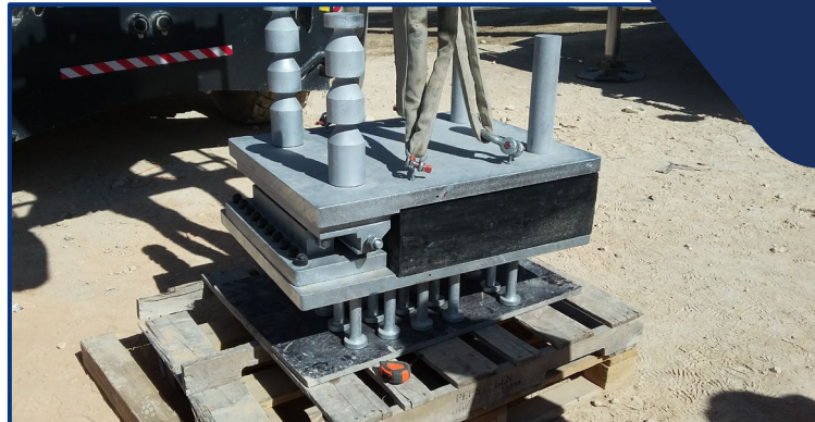
20 MN Press "Compression test"
