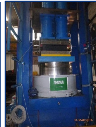
20 MN Press "Compression test"
