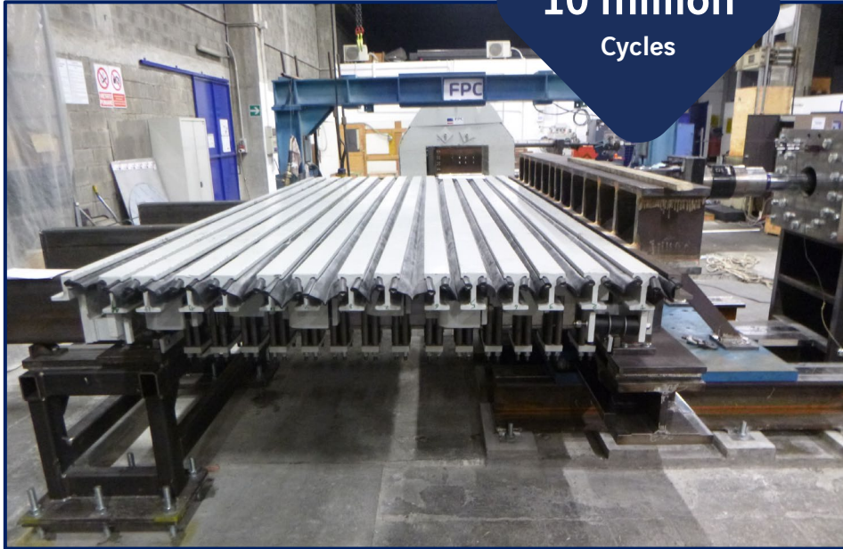
LW (Modular joint) 200 Joints – Qualification for AASHTO Fatigue & load test
