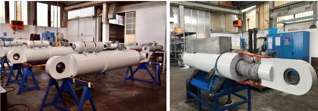
Fig. 12 – ISOSISM® FD 4000/925 during assembly phase
