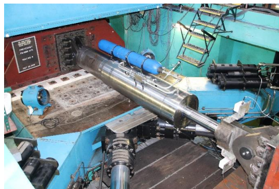
Fig. 10 - ISOSISM® FD 4000/1170 - Qualification test at UCSD lab
