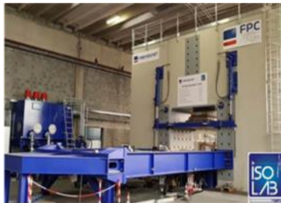
Fig. 6 – The 70 MN ISOLAB® Testing system
