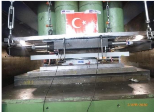
Fig. 15 – Spherical bearing test at ISOLAB and friction test result
